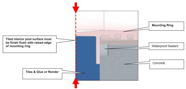
ATTENTION: Interior pool surface must finish flush with the raised edge of the mounting ring, or it will not be possible to properly install the light.
